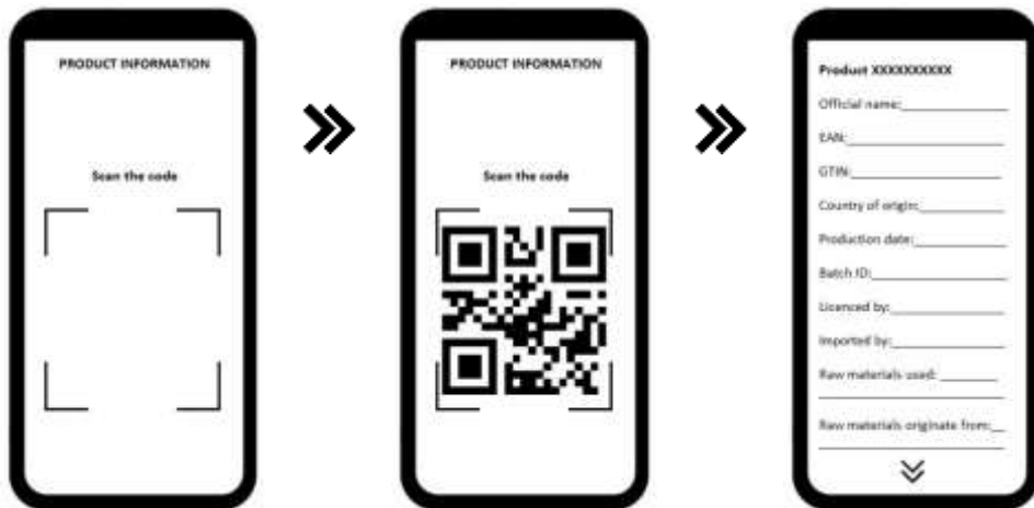
Figure 2. Schematic representation of the process of user interaction with the product-representing QR code using a personal mobile device.
